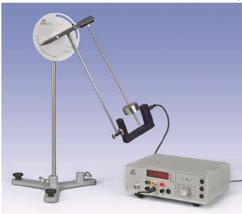
Fig. 1: Variable-g pendulum (photograph and schematic diagram)
