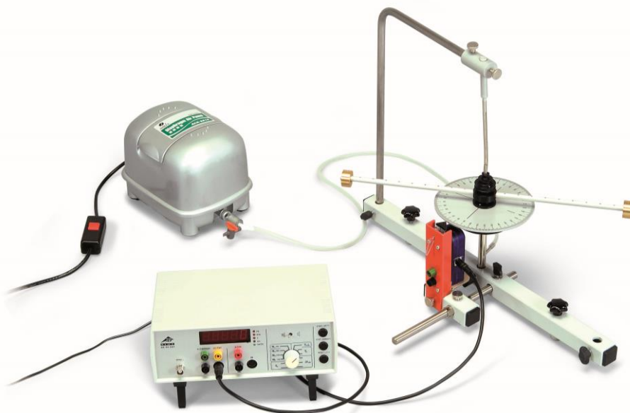
Fig. 1: Experiment set-up for determining the moment of inertia by the torsional oscillation method
