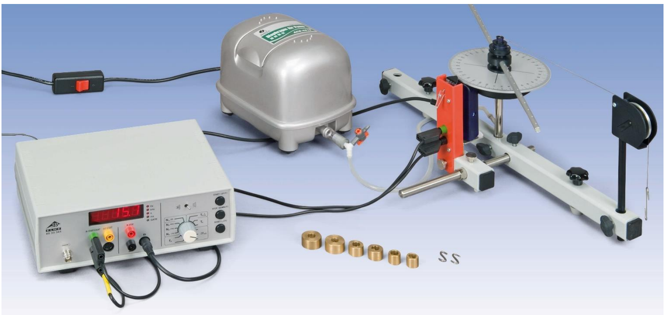
Fig. 1: Experiment set-up for the study of uniformly accelerated rotational motions
