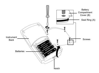
To ensure that the instrument is waterproof:
