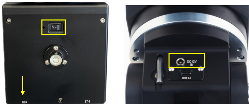
Figure 20. Connecting handset and 12V DC power
