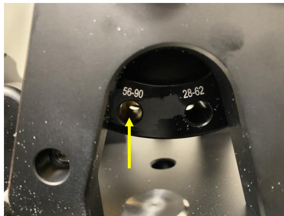
Figure 10. Adjust mount and align the range holes
