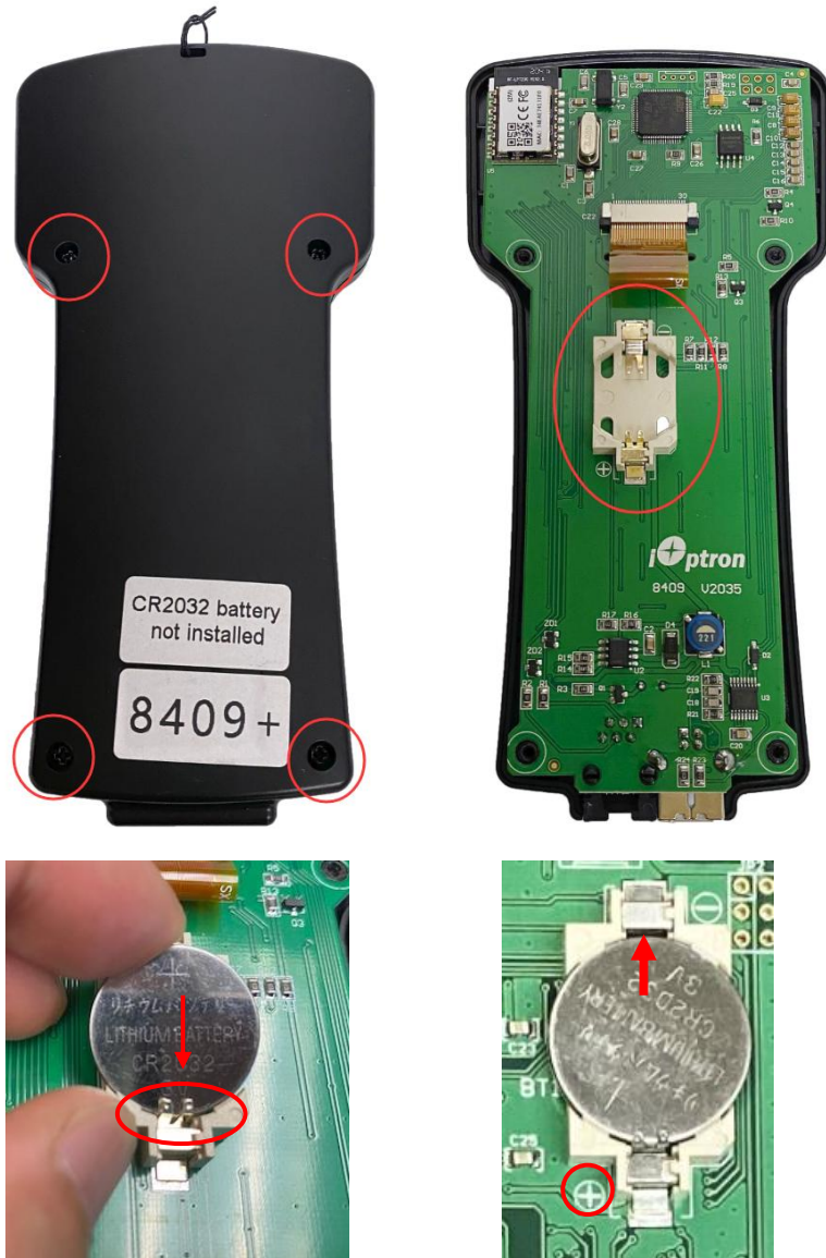
Figure 8. Install a CR2032 battery
