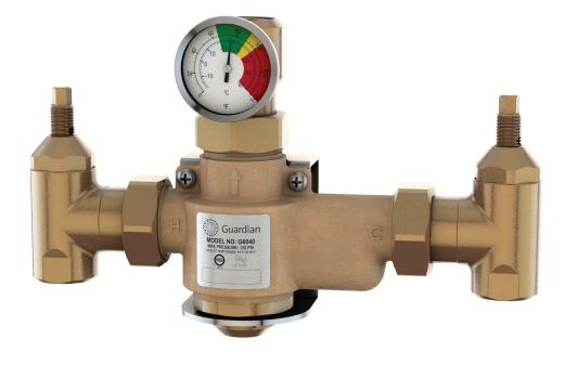
**Application:** Thermostatic mixing valve to blend hot and cold water to deliver tepid water. Valve has flow capacity of 50 gallons (189 liters) per minute at 30 PSI (2.1 bar) pressure drop. Valve can be used to supply emergency shower or combination safety station. Depending on water supply size and pressure, valve can supply multiple units.
